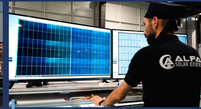
Electroluminescence control in three points.
