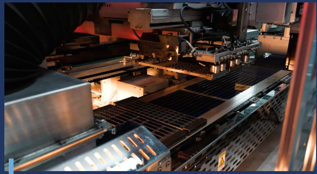
The latest technology allows for cell soldering with machines.
